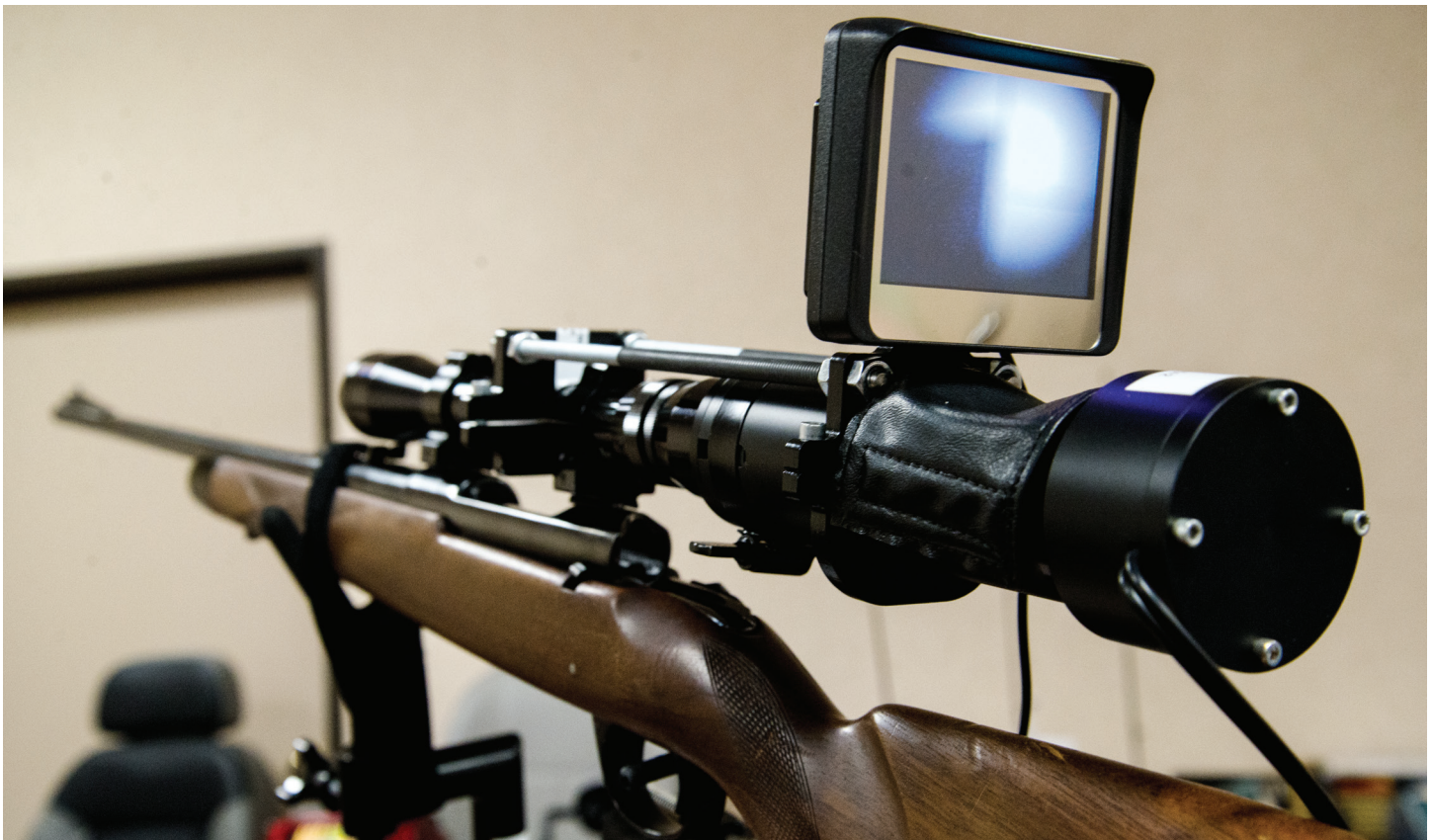
This rifle has been modified with a large screen to help users with limited mobility view the scope from a seated position and fire the trigger with a straw-like apparatus. This entire setup can be mounted onto the arm of a wheelchair.
