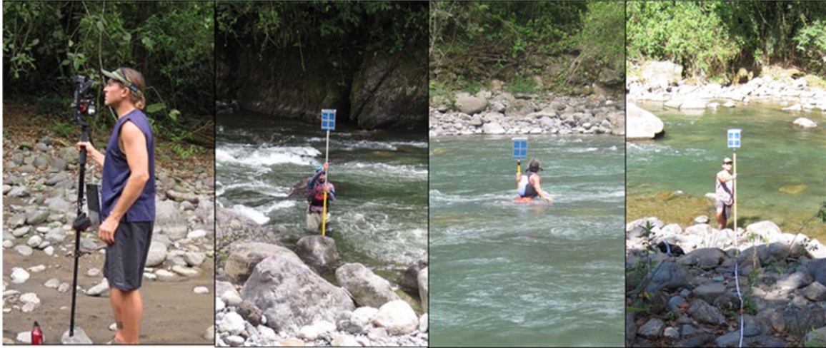
Figure 0-6. Cross section surveys at field sites Bajo Pacuare for San Juaquin, Arriba Pacuare, Tres Equis, and Bajo Pacuare - Laser range finder on stabilizing pole shot at mounted target placard.
