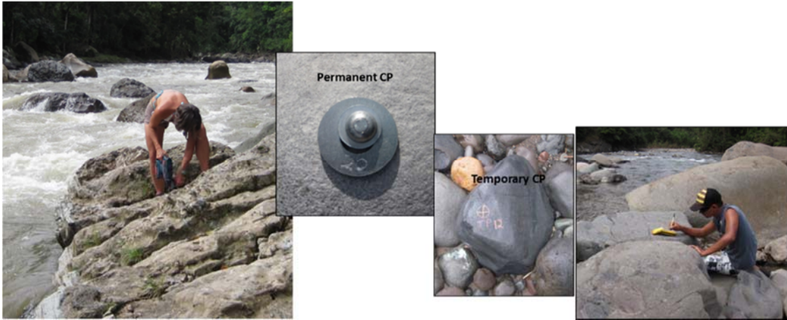
Figure 0-5. Examples of survey control points at field sites. Photos by P.Lind & O. Arroy Nunez.
