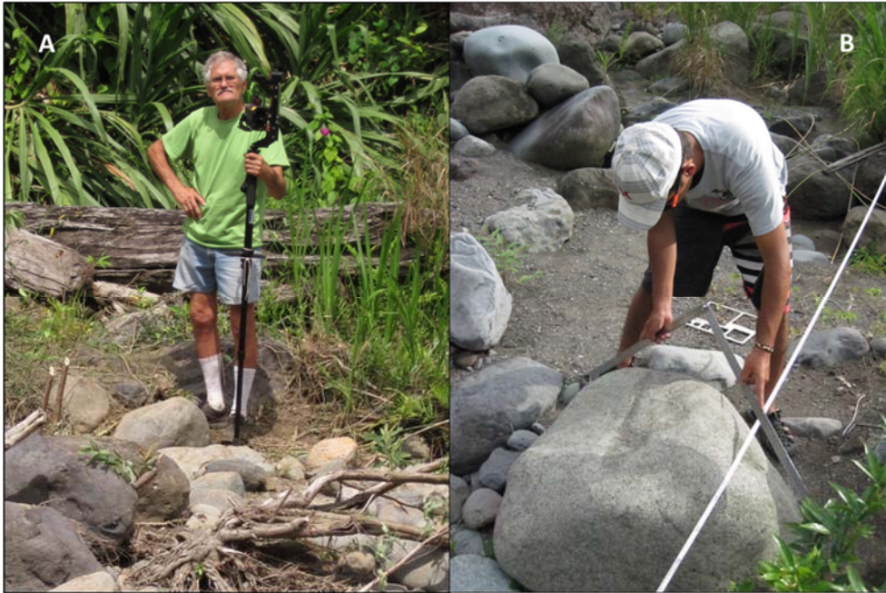
Figure 0-16. A) Laser Range Finder used for cross-section surveys. B) Grain size surveys with calipers and gravelometer. Photos by P.Lind – 2013.
