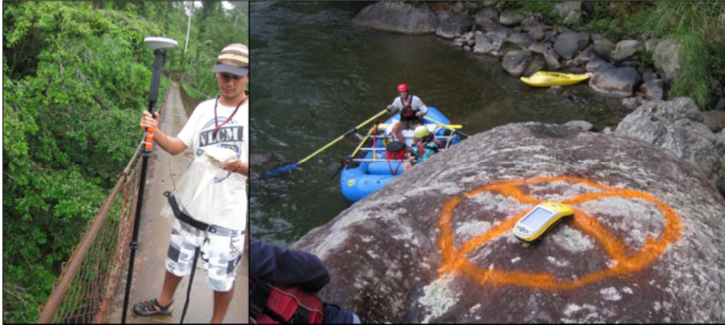
Figure 0-12. Photos of collecting ground control points for SfM model development with Trimble GeoXS and Zephyr antenna on the Rio Pacuare. Photos by P. Lind.
