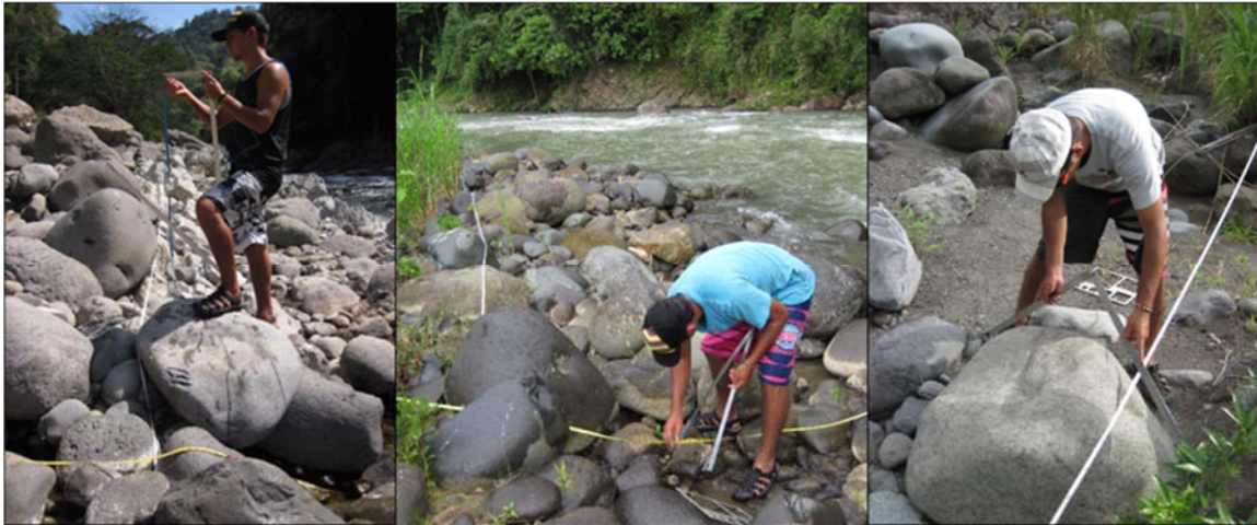
Figure 0-8. Gravel count completed with calipers and gravelometer at field site Tres Equis, Bajo Pacuare por San Juaquin, and Paso Marcos. Photo by P.Lind.
