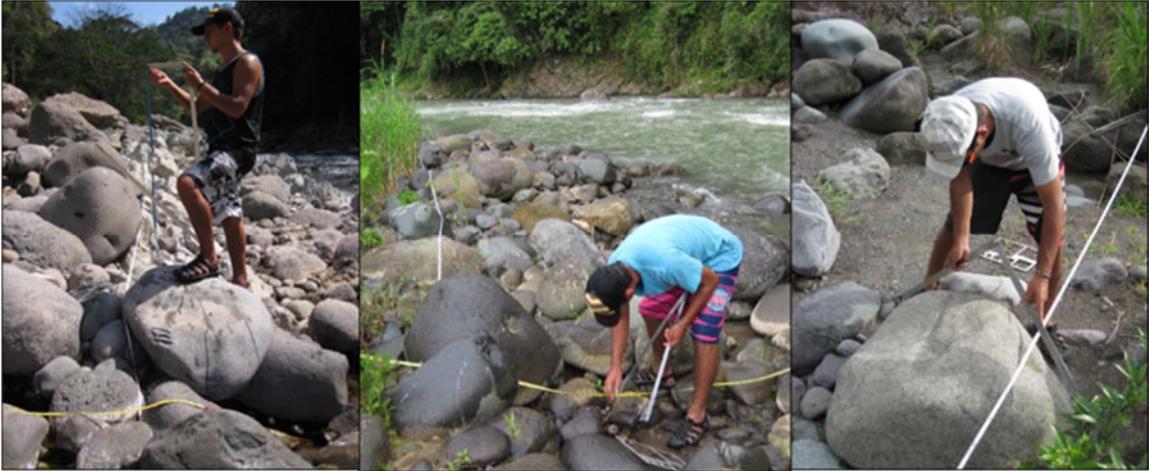
Figure 0-10. Conducting grain-size surveys at depositional bars along the Rio Pacuare (Rkm 62.5, 82.6, and 74.9). Photos by P. Lind.
