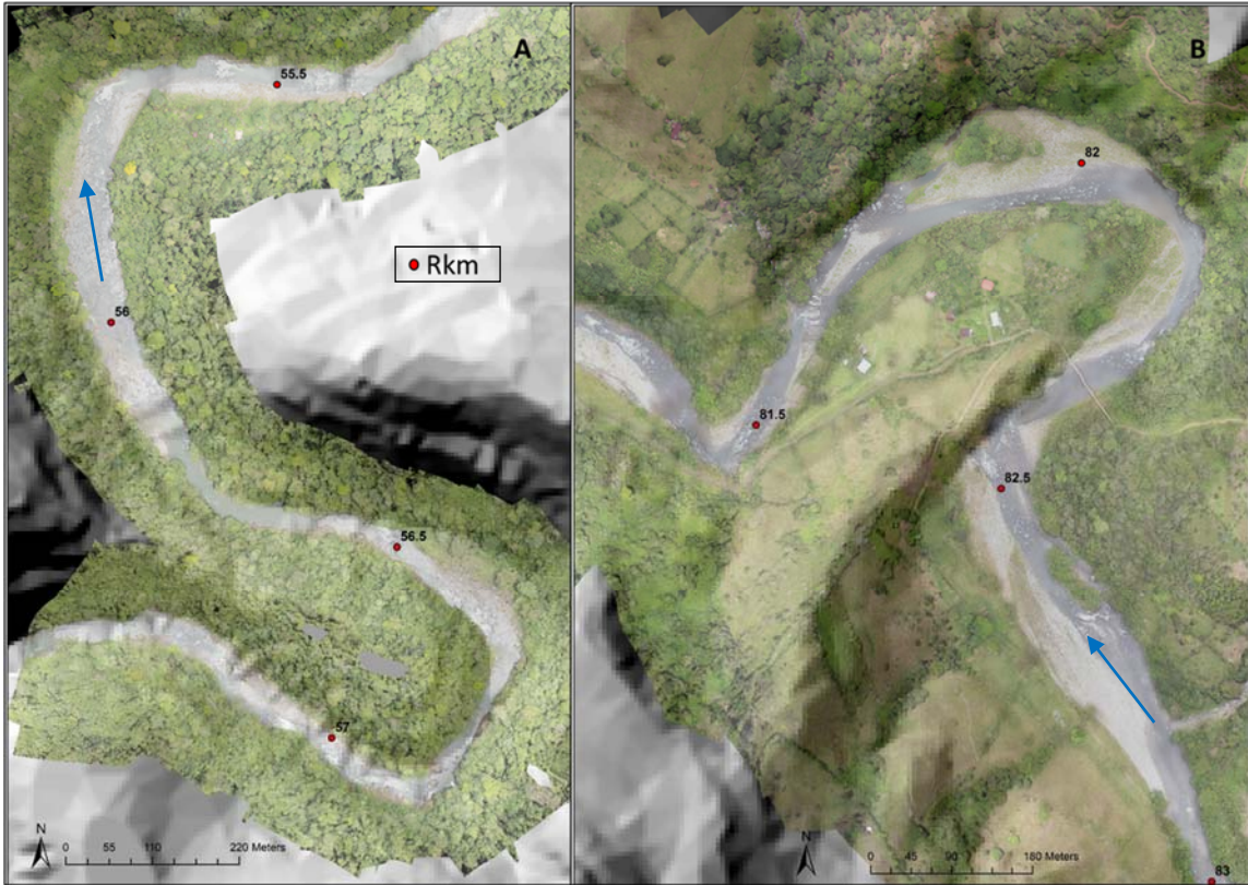
Figure 0-22. Aerial images of channel deflection (bedrock controlled meandering) at (A) Rkm 57 and (B) Rkm 82.
