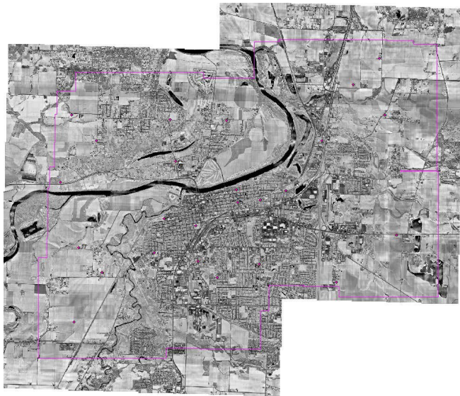
Tutorial 13: GCP spread around the LIDAR Intensity image that can now be used as Markers in PhotoScan or Validation Points for error assessment.
