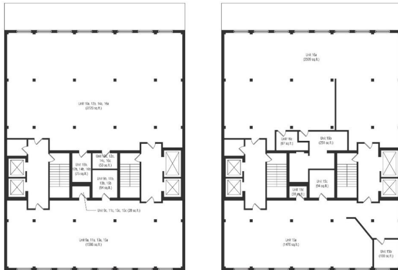
Figure 520, 521 (left to right): Building 17, seventh floor (1915); same floor (1984); 1" = 32'. North is down.
