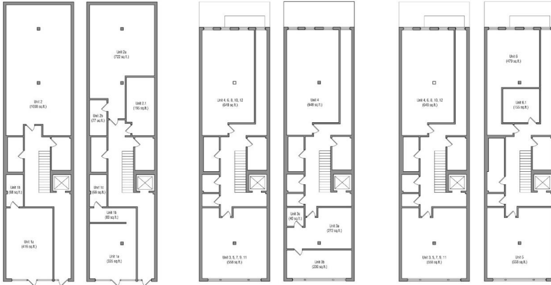
Figure 408, 409, 410, 411, 412, 413 (left to right): Building 14, first floor (1911); same floor (1980); second floor (1911); same floor (1980); third floor (1911); same floor (1980). 1" = 32'. North is down.
