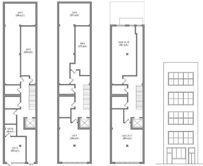
Figure 146, 147, 148, 149 (left to right): Building 5, first (ground) floor (1930); second floor (1930); floors 3–5 (1930); street-front elevation (1974). For plans, north is down.
