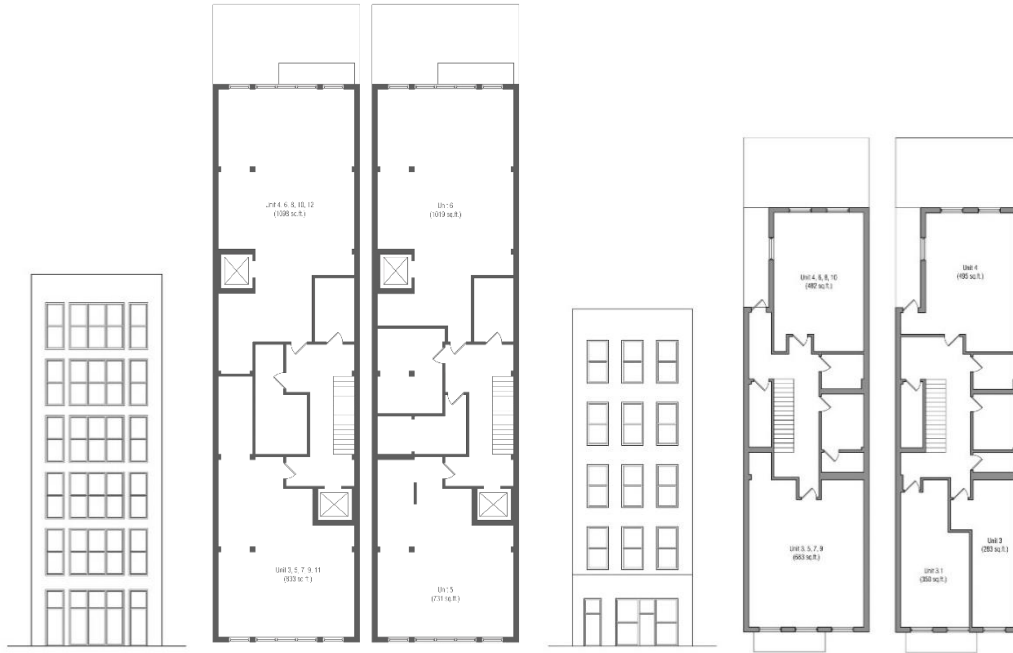
Figure 660 (left to right): Elevation of Building 20 (1978); third floor plan of Building 20 (1916); same floor (1978); elevation of Building 9 (1974); second floor plan of Building 9 (1930); same floor (1974); 1" = 32'.
