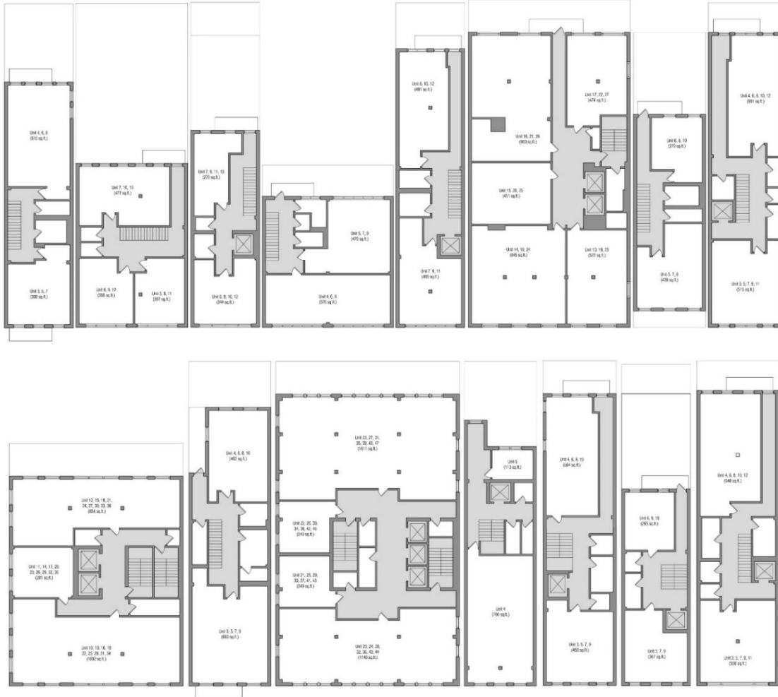
Figure 656 (left to right): Initial plans of buildings 1-7, 15 (top row) and 8-14 (bottom row) with core areas highlighted in dark tone. 1" = 32'. Plans oriented so that the street front would be down.
