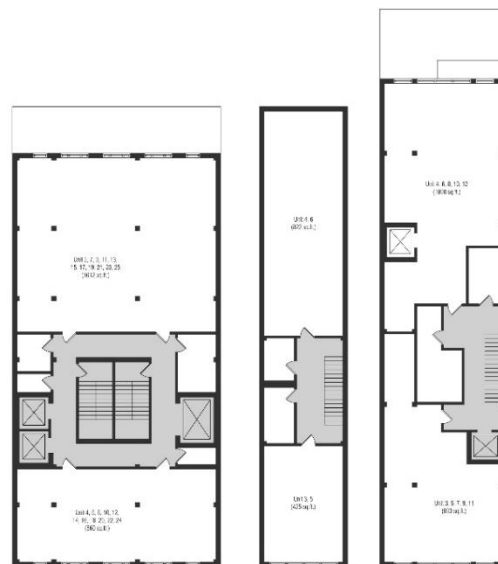
Figure 639, 640, 641: Plan of Building 18 (left), Building 19 (middle), and Building 20 (right), with core areas highlighted in dark tone. 1" = 32'. Plans oriented so that the street front would be down.
