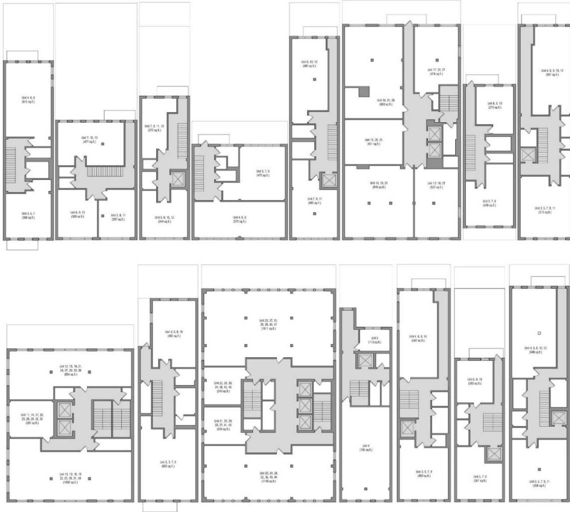
Figure 458 (left to right): Initial plans of Buildings 1-7, 15 (top row) and 8-14 (bottom row) with core areas highlighted in dark tone. 1" = 32'. Plans oriented so that the street front would be down.
