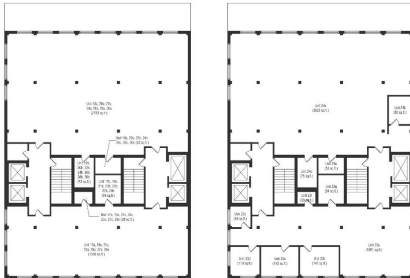
Figure 528, 529 (left to right): Building 17, eleventh floor (1915); same floor (1984); 1" = 32'. North is down.
