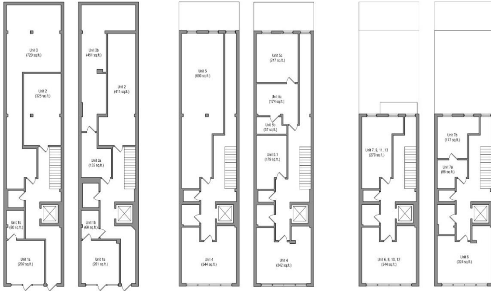
Figure 103, 104, 105, 106, 107, 108 (left to right): Building 3, first floor (1925); same floor (1980); second floor (1925); same floor (1980); third floor (1925); same floor (1980). 1" = 32'. North is down.
