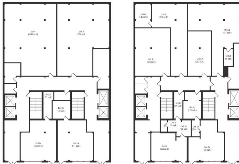
Figure 508, 509 (left to right): Building 17, first (ground) floor (1915); same floor (1984); 1" = 32'. North is down.
