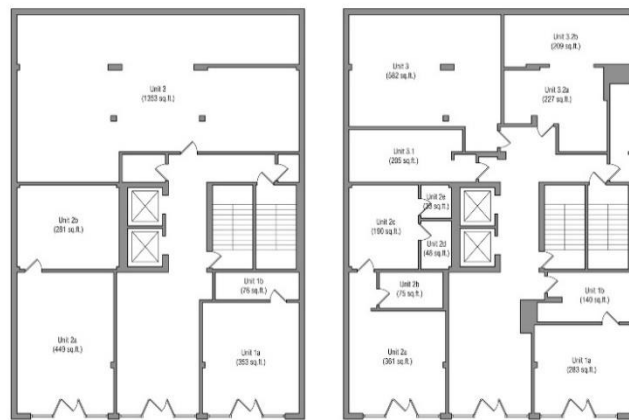
Figure 228, 229 (left to right, top down): Building 8, first floor (1926); same floor (1981). 1" = 32'. North is to the left.
