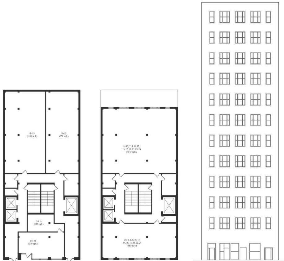
Figure 547, 548, 549 (left to right) Building 18, first (ground) floor (1910); floors 2–12 (1910); (right) street-front elevation (1981). 1" = 32'. For plans, north is up.
