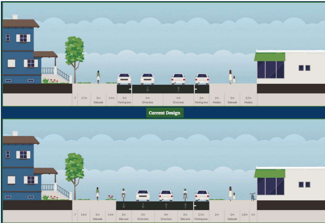
Figure 46: Jackson Street infrastructure and street area measurements.
