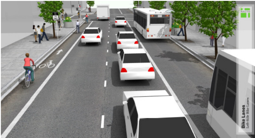
Figure 52: Left-Side Bicycle Lane
