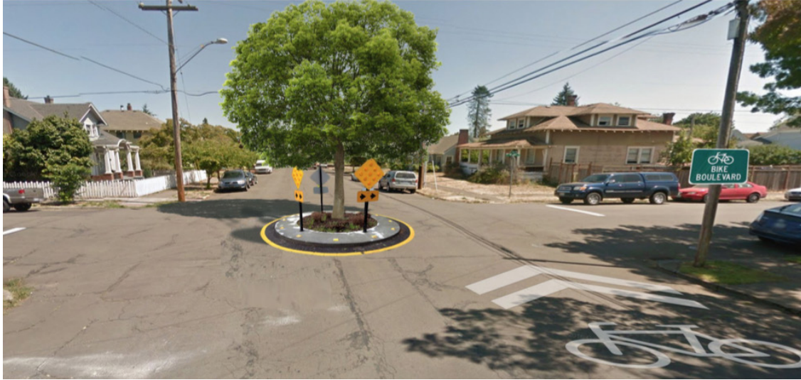
Figure 47: The addition of islands at smaller intersections is a traffic calming device and is beneficial for cyclists.
