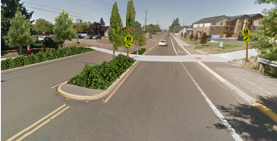
Figure 5: An example of what the addition of an Island might look like on Queen Avenue.
