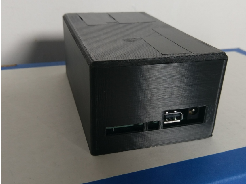
Figure 3.1: A side-view of the shell shows cut-outs for USB connections & power supply.
