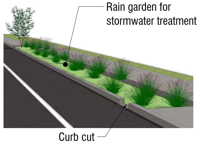
Option: Stormwater Facility
