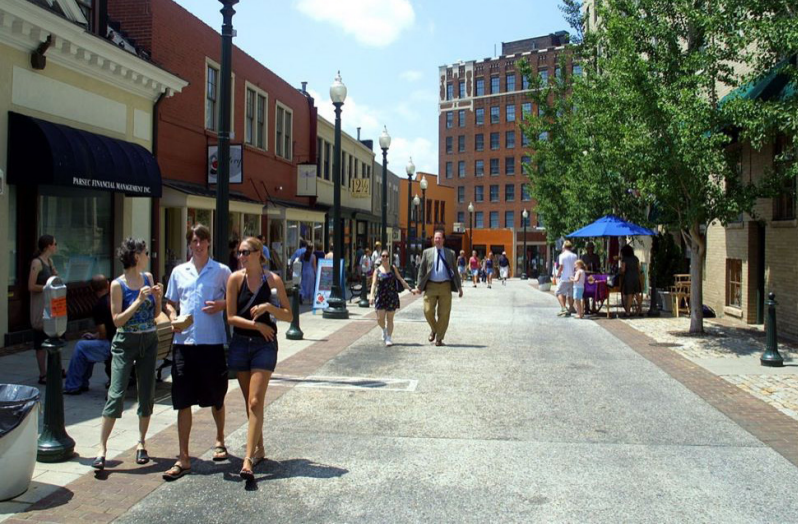
Figure 33: Shared streets are designed for all modes to mix, with pedestrians setting the pace.
