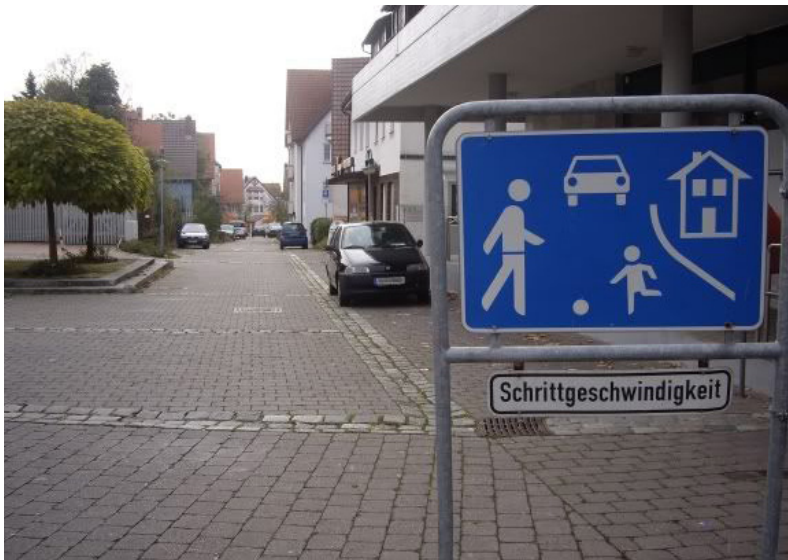
Figure 32: Shared streets are designed for all modes to mix, with pedestrians setting the pace.
