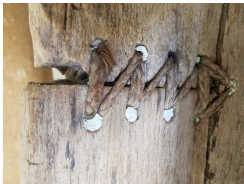
Figure 5: A preserved Marquesan near-shore fishing canoe showcases the typical manner of lashing planks flush to one another with fiber rope and bread fruit caulking.
