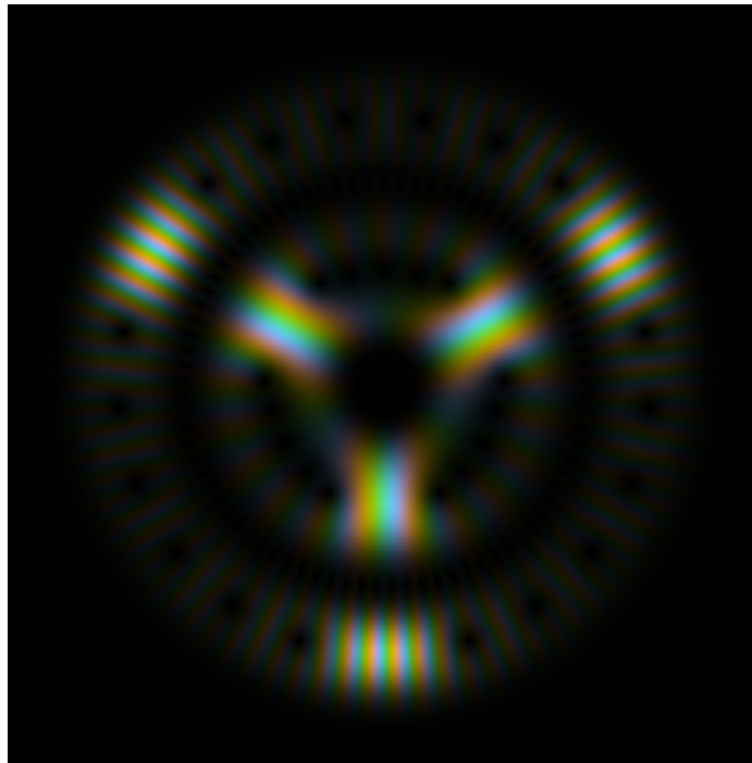
FIGURE 5.6: Representation of the complex amplitude for the beam given in Equation 5.4. This beam has an inner and an outer portion that rotate in opposite directions as the beam propagates through focus.
