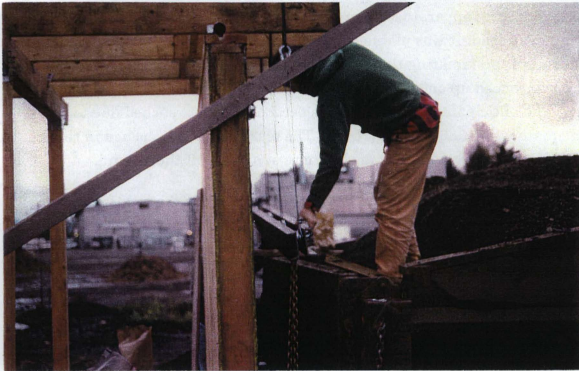
Figure 4-5, Exterior Bearing Wall Load Test
