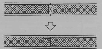
• Shiplap joints reduce installation by 20%, improve air tightness and reduce fasteners by one half.
