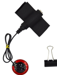
Figure 80: Photo of contact microphones used in Brigit
