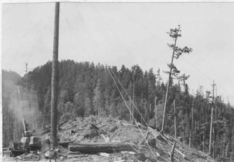
Figure 57. Large Scale Logging (high-lead yarding). Logs are yarded from the forest by cable and donkey engine (above) to a collection point near the spar pole (below). Here, using a logging arch (bottom left), the logs are loaded onto waiting trucks.
