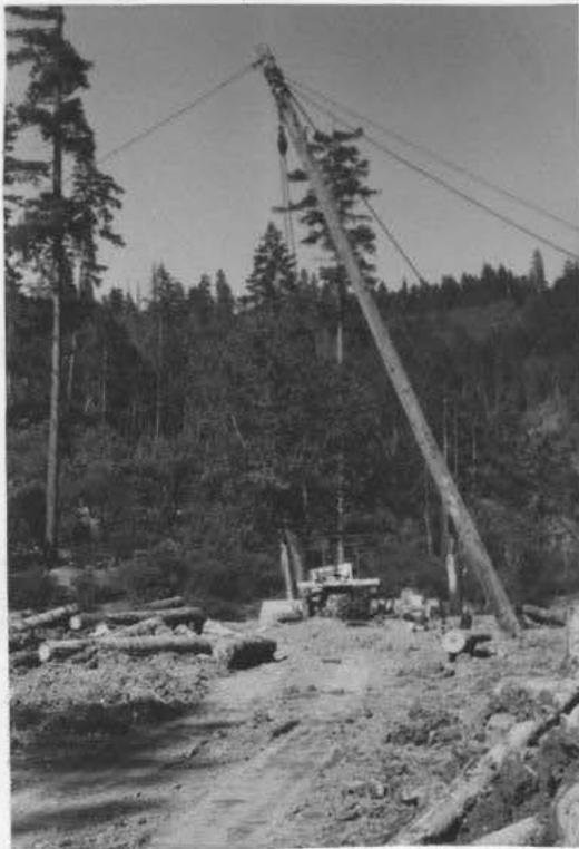
Figure 58. Small Scale Logging (ground yarding). Logs are skidded from the forest by caterpillar tractor (above) to a point where a gin pole (below) has been reared. Here, using the winch on the tractor and a block and tackle system, the logs are loaded onto trucks.
