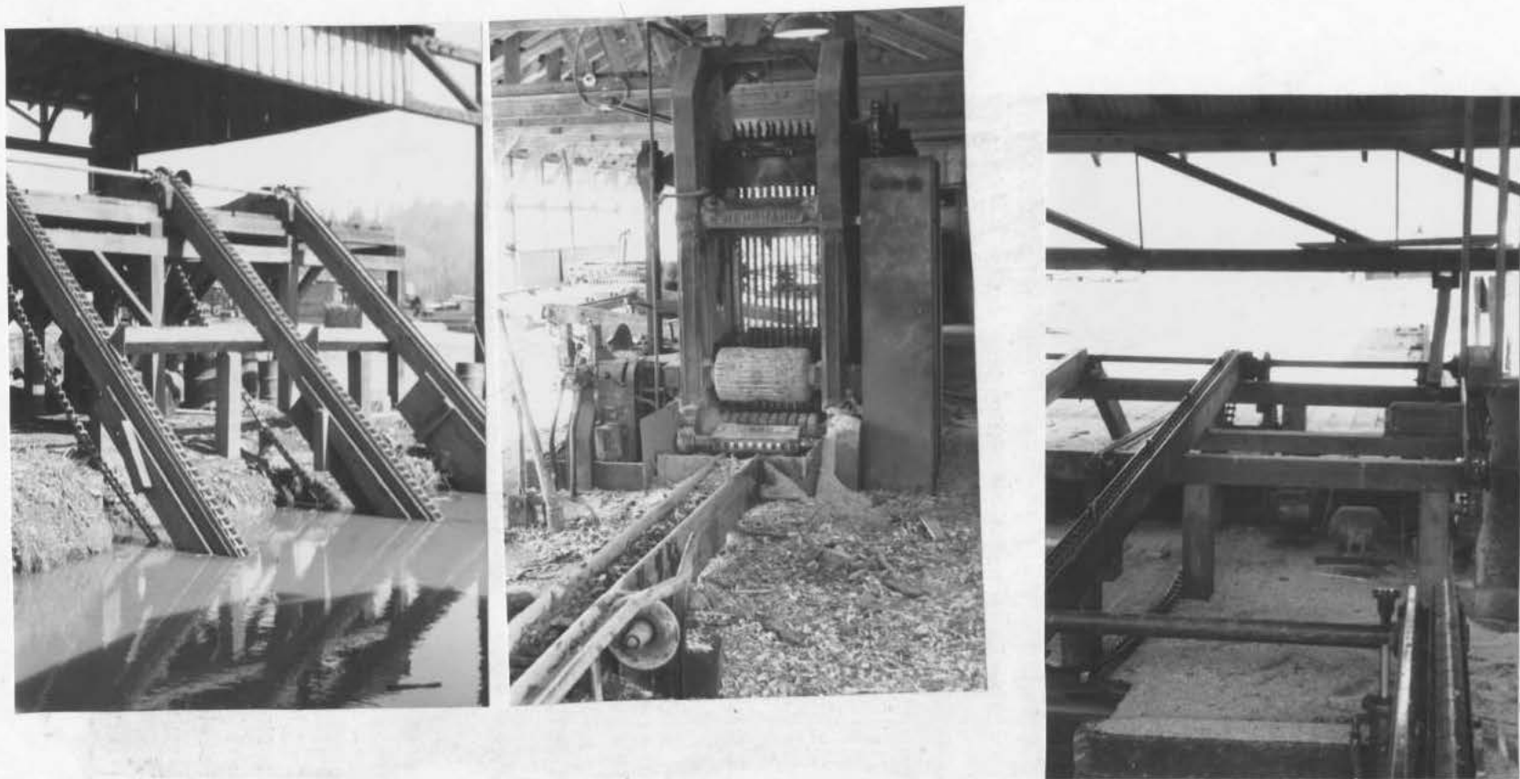
Figure 60. LEFT: Rotating chains carry logs from the pond into this small, but efficient sawmill in Wolf Creek. MIDDLE: German gangsaws are, here, set for 2 inches. These saws make the first cut since there is no headsaw in the mill. Resaws may be seen in the left rear. RIGHT: Trimmer saws pictured here, make the final end cuts and the rough lumber is then carried on the "green chain" (background) to the end of the dock where it is stored or loaded.
