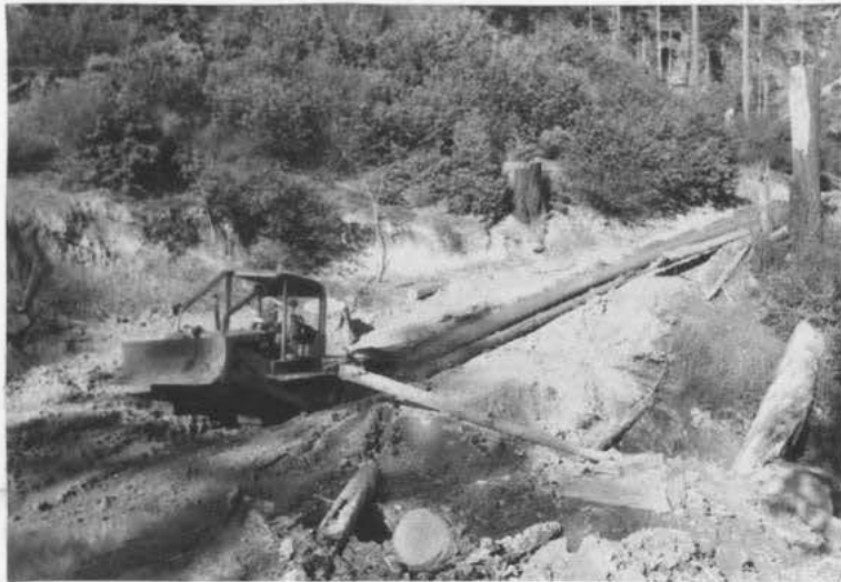
Figure 58. Small Scale Logging (ground yarding). Logs are skidded from the forest by caterpillar tractor (above) to a point where a gin pole (below) has been reared. Here, using the winch on the tractor and a block and tackle system, the logs are loaded onto trucks.
