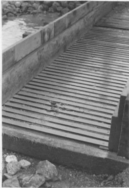
Figure 26. Speaker Placer. Gold-catching riffles in sluice are made of steel to resist wear.
