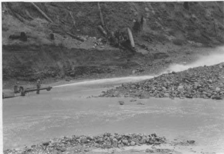
Figure 22. Hydraulic mining on Wolf Cr. At the left center is a miner directing wash material with a giant, toward a sluice located off the photo at the right.
