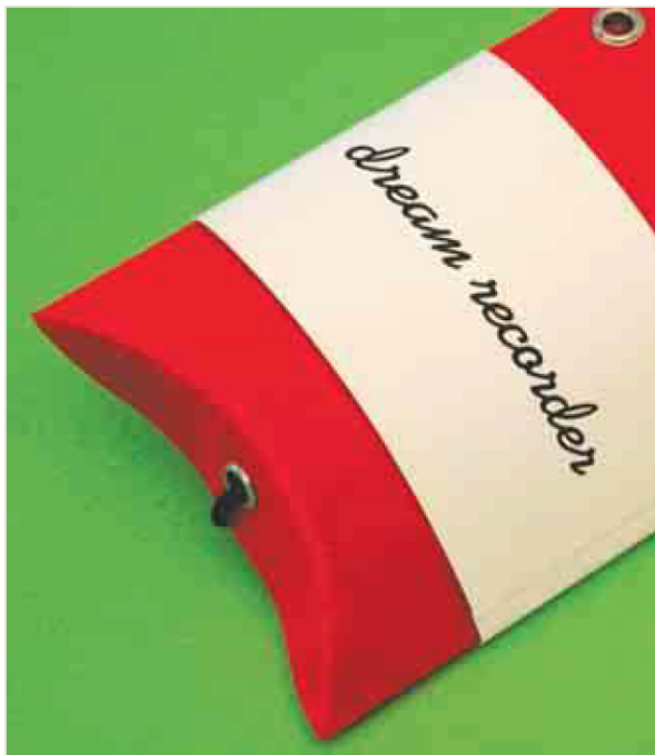
Figure 15. A “Dream Recorder.” Note. Participants were asked to record dreams they had during the night. Pulling the cord on the device would give participants 10 seconds to record their dreams (Gaver et al., 2004).
