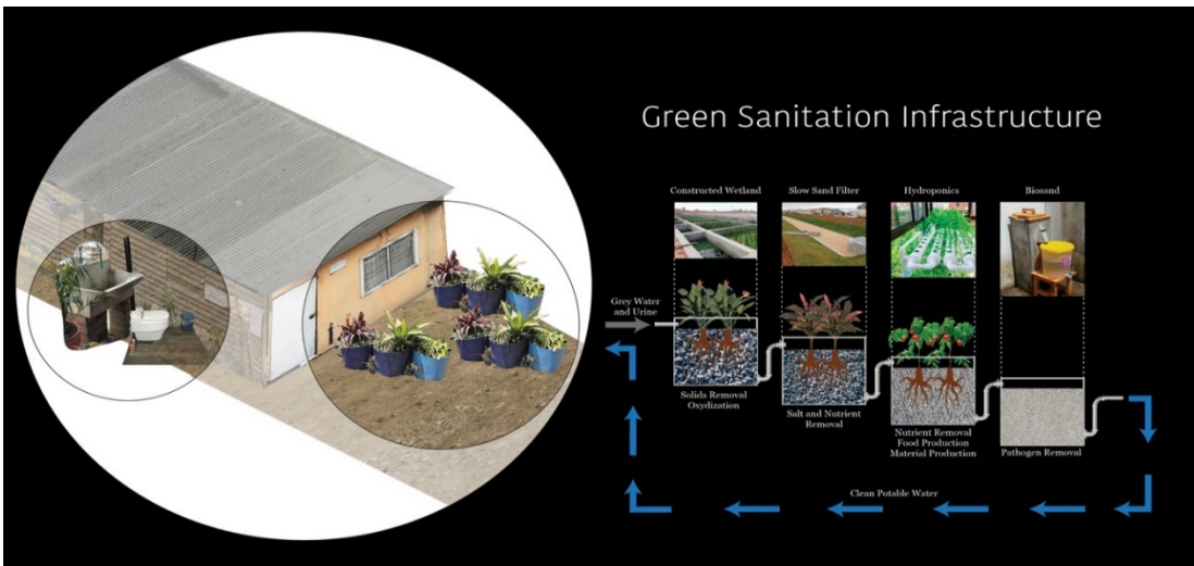
Figure 44. Most recent design of green sanitation infrastructure.
