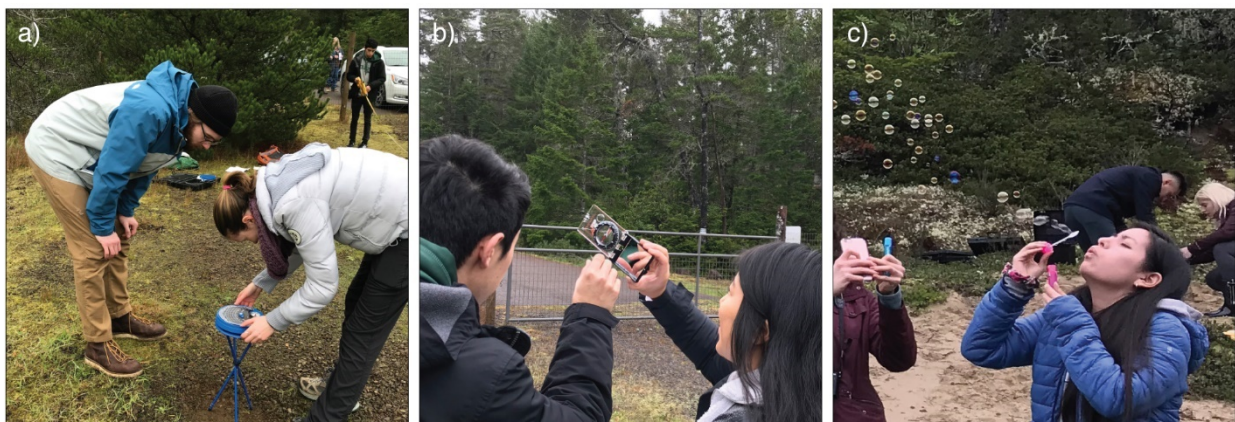
Figure 1. (Dunes City) Solar site surveys include the use of a) solar pathfinders to document site shading; b) inclinometers and field tape measures to establish the heights and positions of site shading elements for use in computational models; and c) airflow bubbles to document prevailing wind directions on the site.
