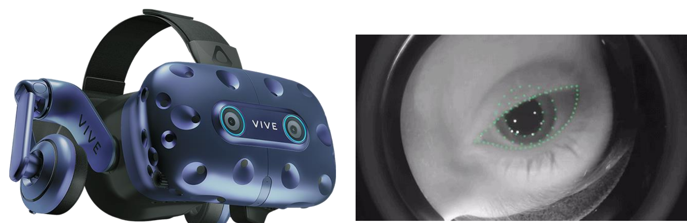
Figure 1. The VIVE Pro Eye VR Headset used (left), and an example of the cameras within the headset tracking an eye.
