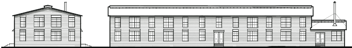
Figure 1.6. 1917 Quartermaster General 600-series design for mobilization barracks. Graphic created by the author.
