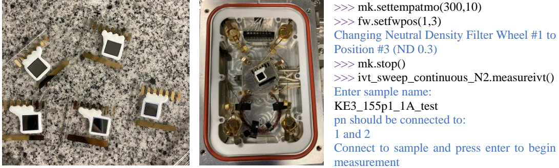
Figure 36. Steps for testing IBC devices. Completed devices (left), device being tested in the stage (center), and commands and code responses in device testing in Python Shell (right). See Appendix B for Python code text.
