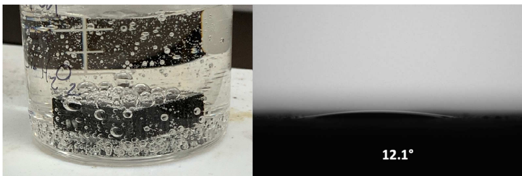
Figure 3.8 PG sample soaking in oxidizing solution (left) and subsequent contact angle(right).
