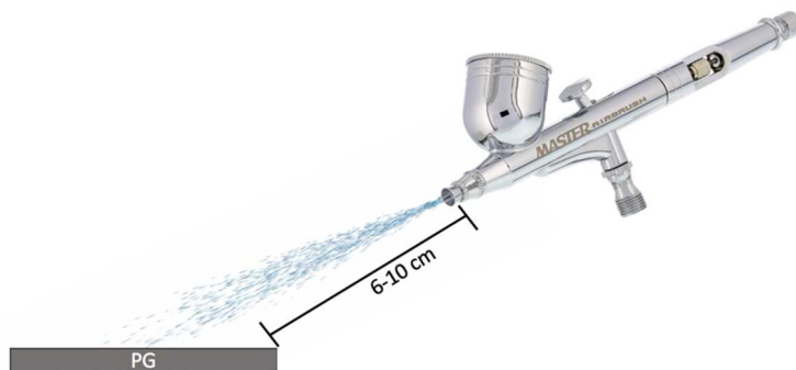
Figure 3.22 Schematic depicting airbrush used for spray coating fabrication.
