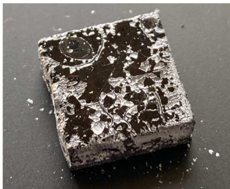
Figure 3.12 Sample showing large scale cracking of \text{Al}_2\text{O}_3 after attempt to coat via sol-gel method.
