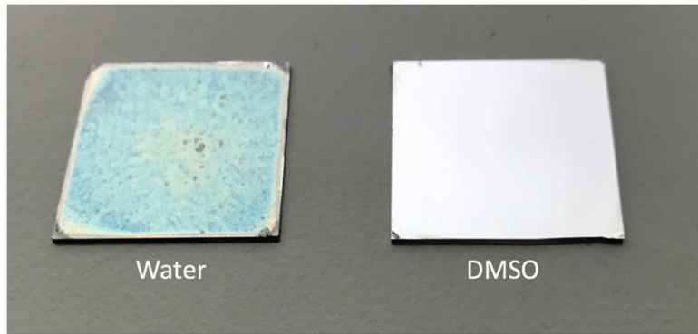
Figure 2.3 CoAl films fabricated from water (left) and DMSO (right). After spin coating and soft bake at 250 °C films from water had significant surface defects compared to ones from DMSO.
