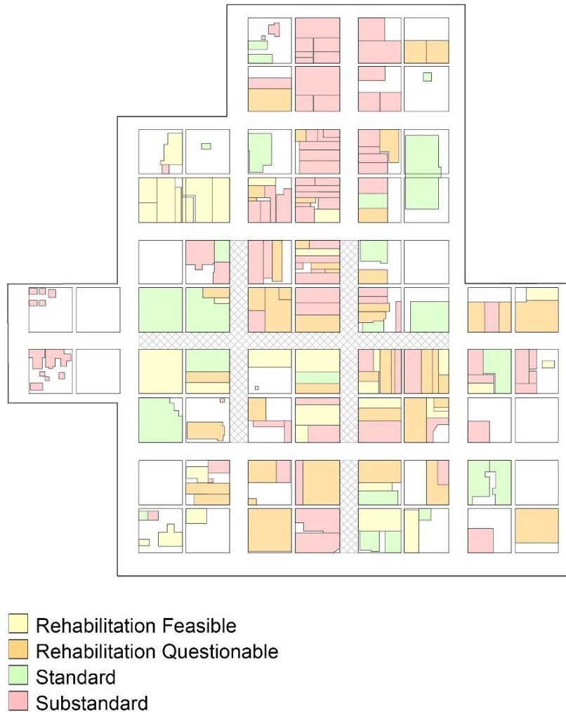
Figure 5.13. A map showing the structural condition of CEP area buildings before the renewal.
