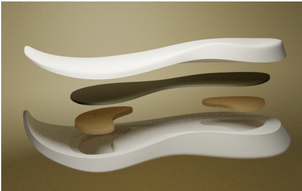
Figure 35. Proposed layering of the flax shank displayed in CAD.
