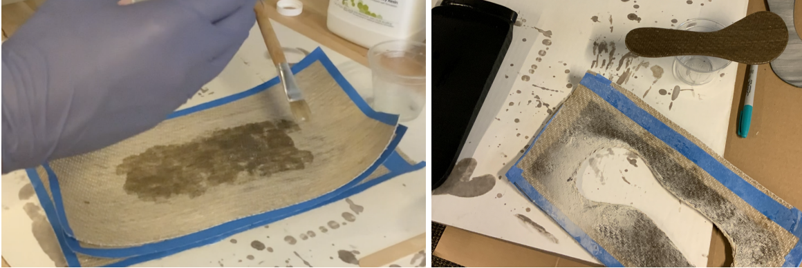
Figure 36. Custom flax fiber lay up process, material cutting, and finishing.
