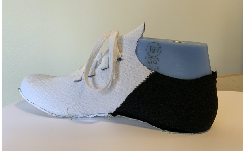
Figure 33. One of the more finalized upper prototypes made in tandem with the 3D model.
