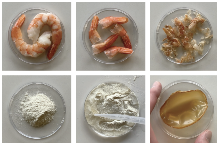
Figure 30. Development process of chitin bioplastic from shell to plastic mold.
