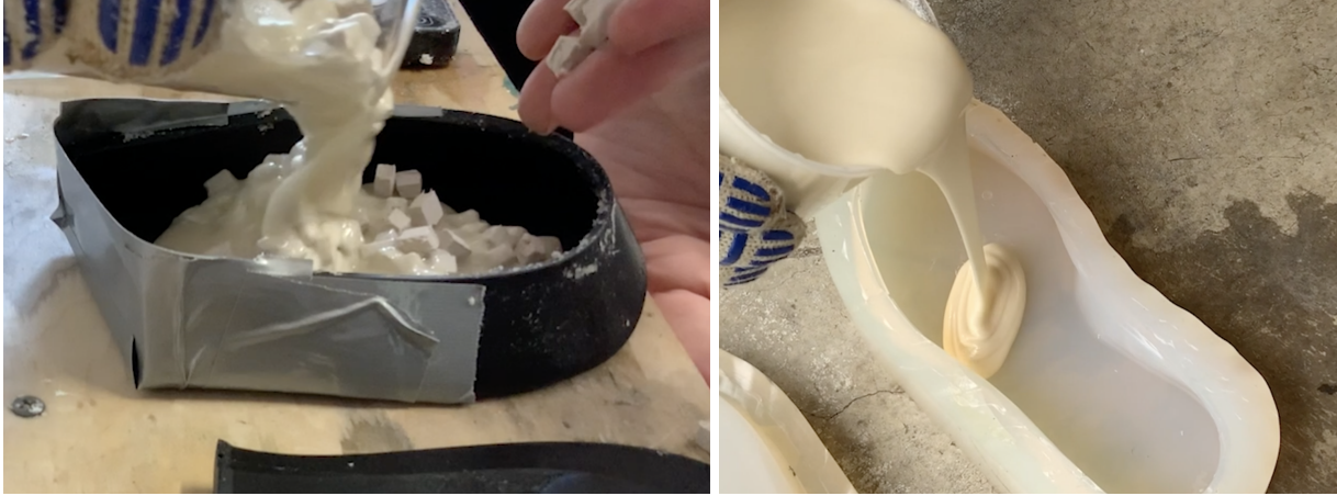
Figure 40. Midsole exploration and foam integration to influence material hardness.
