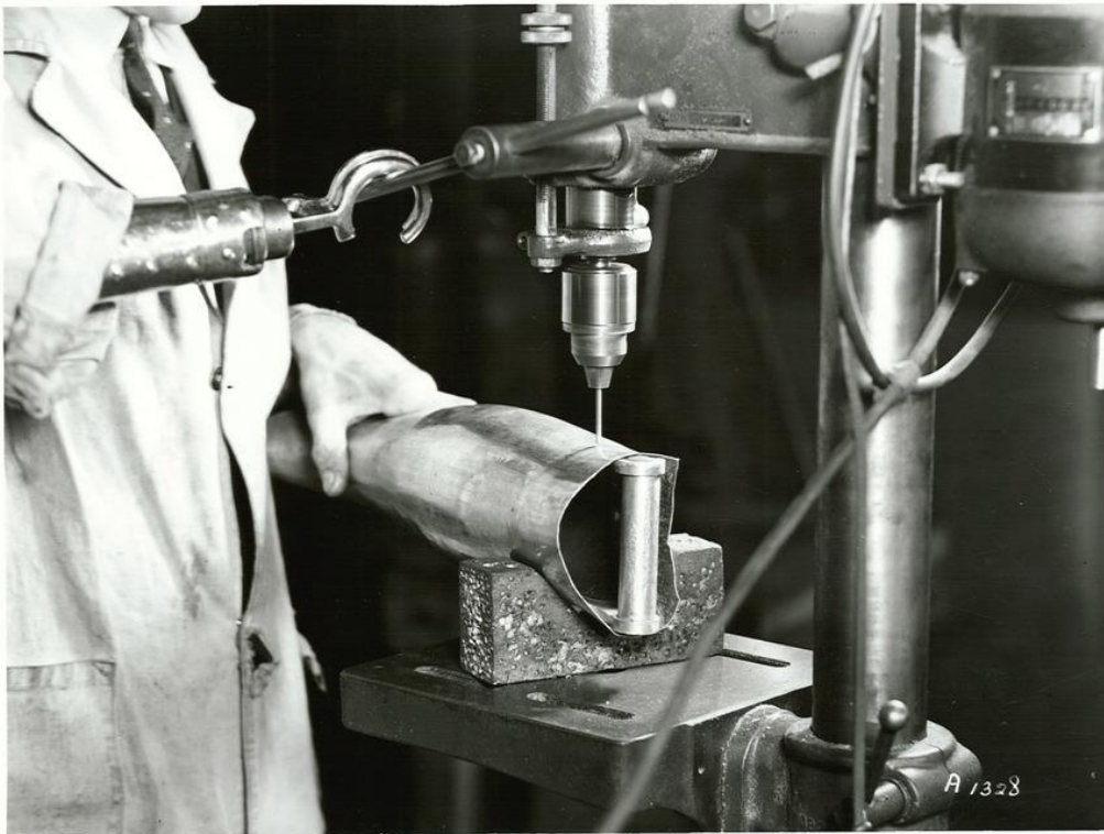
Figure 9: A man with a mechanical arm constructing a prosthesis with the aid of a drill press
