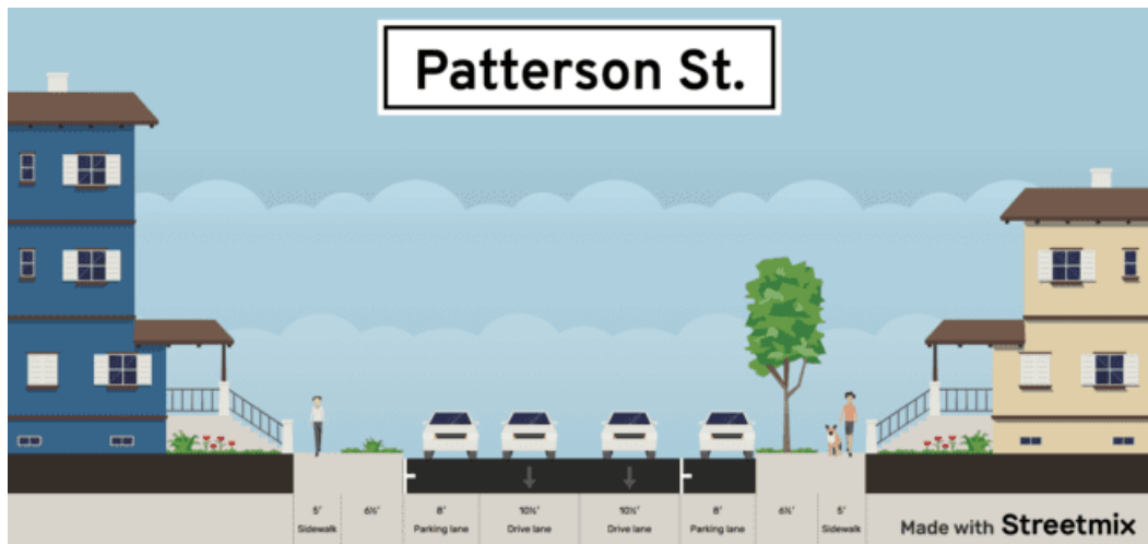
Figure 4. Right-of-way allocation on Patterson St.
