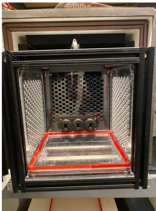
Figure 8. Image of the inside of the inner box and the three water ports
