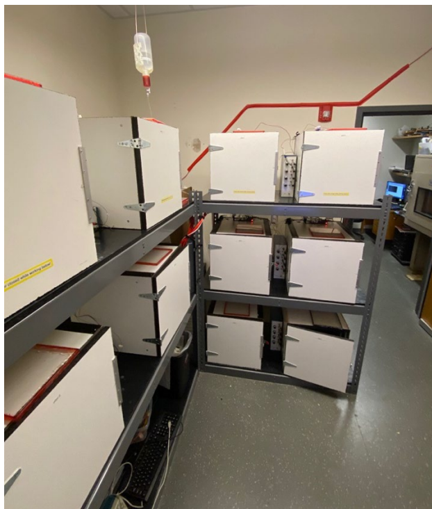
Figure 6. Ten sound attenuating chambers, optic
