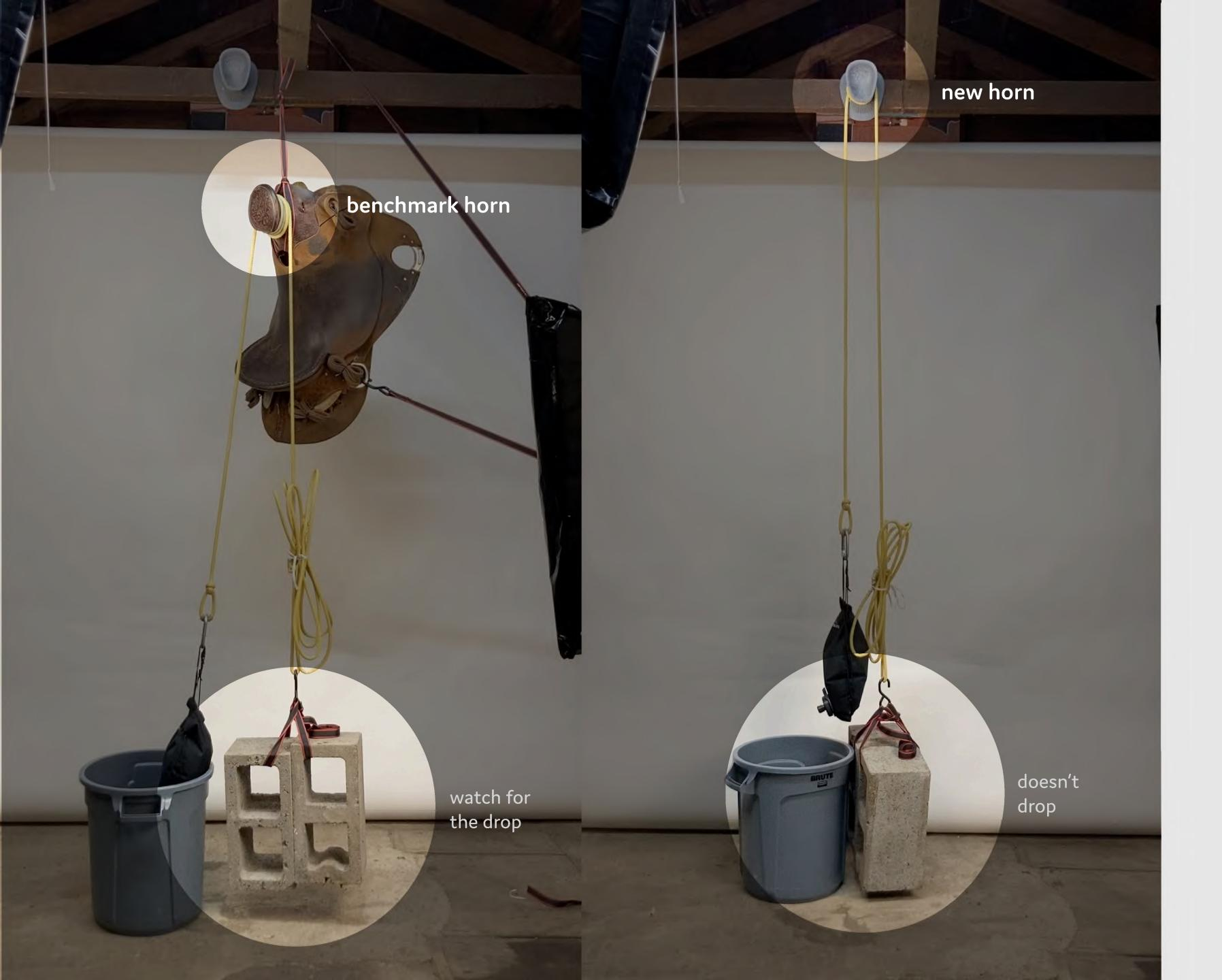
Benchmark horn coefficient of static friction:
