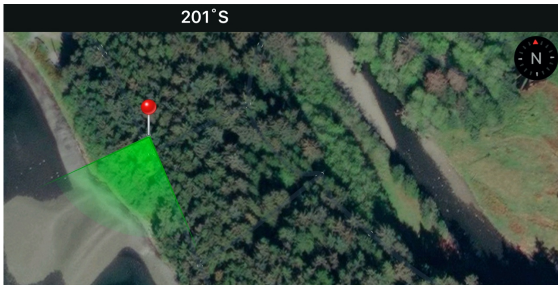
Figure 5-14. Geospatial context for Solocator snapshot approximating S-01 camera station, linked with the previous figure. Close examination of application-generated points in field conditions indicates varied positioning accuracy, in this case on the order of a ~2m margin of error.
