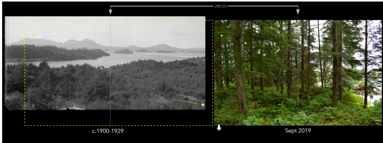
Figure 6-12. Rephotographic pairing for S-10, including overlays detailing selected reference points. Fence alignment is visible at lower right, roughly parallel to Ehrler Street today. Lens center bears approximately 294°W-NW(T), logged 57° 3' 11.0118", 135° 20' 17.289"W. Note: the following figure shows the same views, superimposed. (SITK 26289)
