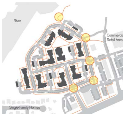
Figure 7. A distribution of access points allows direct movement and connection to a number of different areas, including streets and a nature trail. Typical developments incorporate only a single connection to an arterial or collector street.
