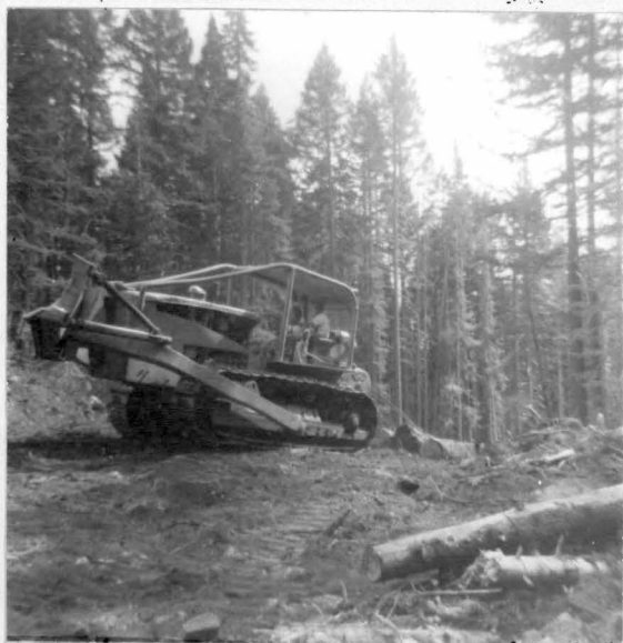
Fig. 39.--Caterpillar Tractor Skid- ding Logs. Tractor is equipped with winch and bull-dozer.
