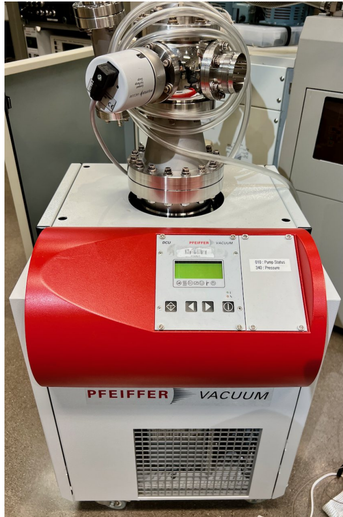
Figure 3.24. The auxiliary pump
