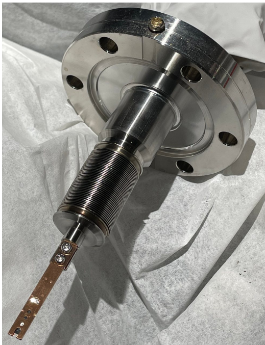
(a) The aperture removed from the instrument (b) Close-up of the aperture holder; the aperture strip is the dark insert at the top behind the holes
