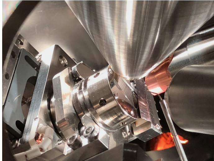
Figure 3.11. A view into the main chamber. The objective lens is the triangle at the top; the SEMPA input optics are the copper colored bit right center; and the Micro Ion Etching Device (MIED) is darker silver cylinder to the right.
