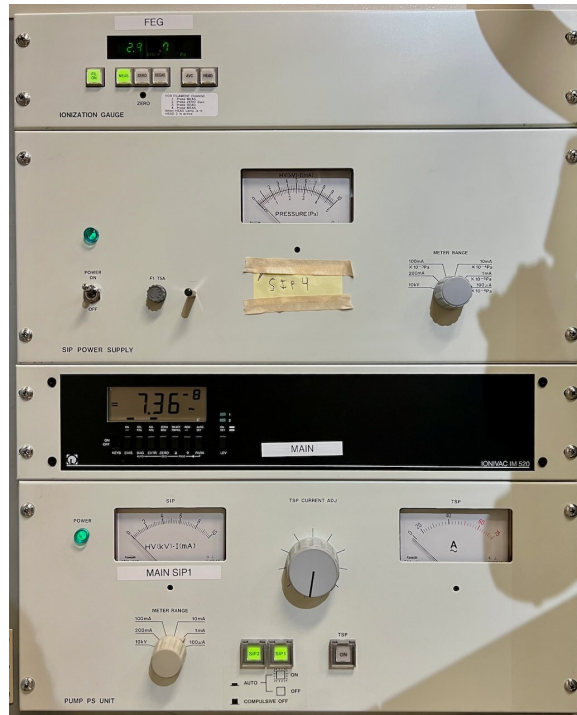
Figure 3.6. The pressure in the FEG is shown on the top gauge; units are Pa
