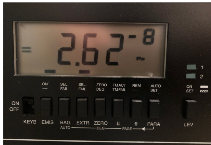
Figure 3.12. The pressure gauge for the main chamber; units are Pa
