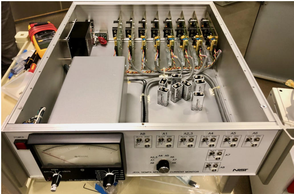
Figure 13.6. This unit houses 8 nanoammeters, each on a separate card
