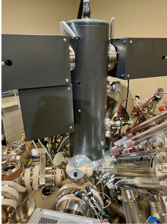
Figure 3.8. 3 of the 5 SIPs are visible as grey boxes on the sides of the electron column
