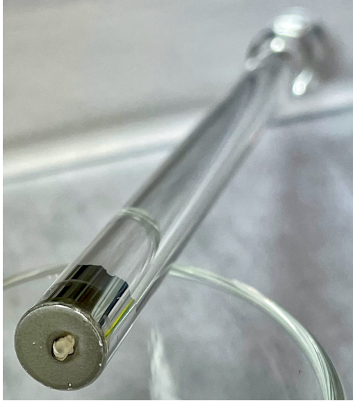
(a) A light pipe with the phosphor burned in the center
