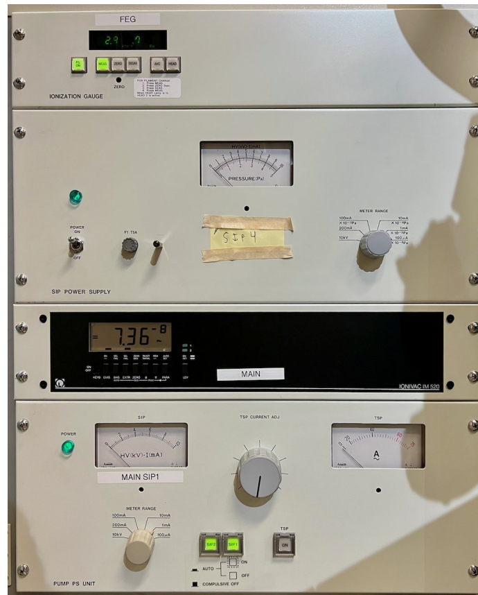
Figure 3.9. The currents for SIP 1 and 4 are shown on the fourth and second gauges, respectively
