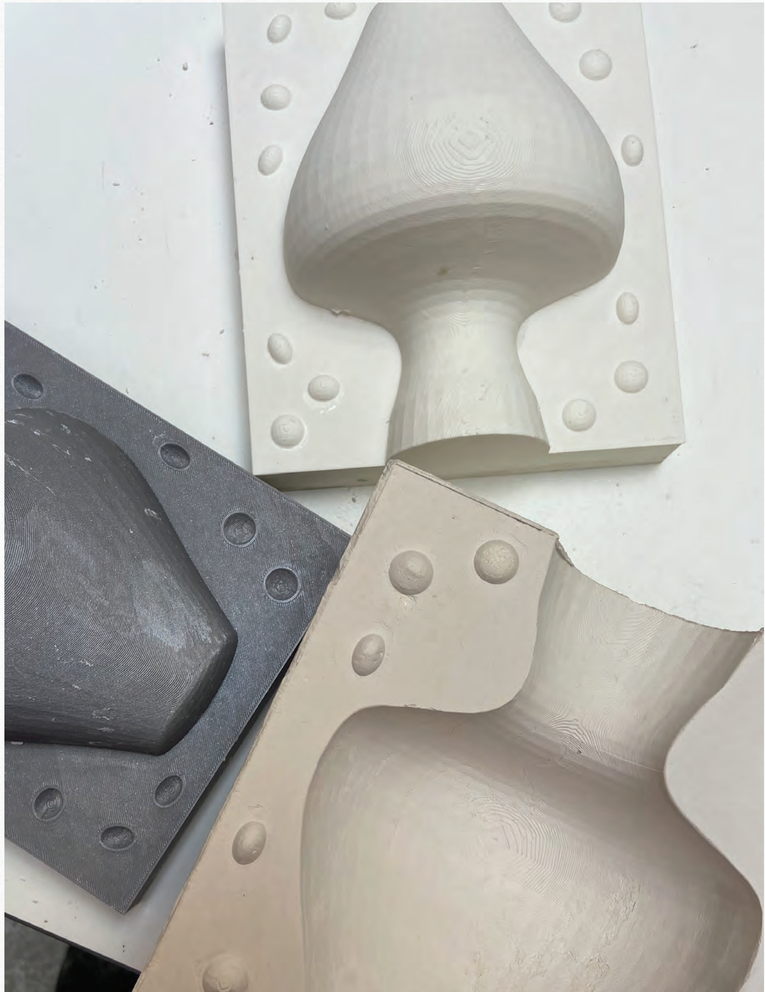
The step-by-step process of utilizing the 3D print to create the master mold.
