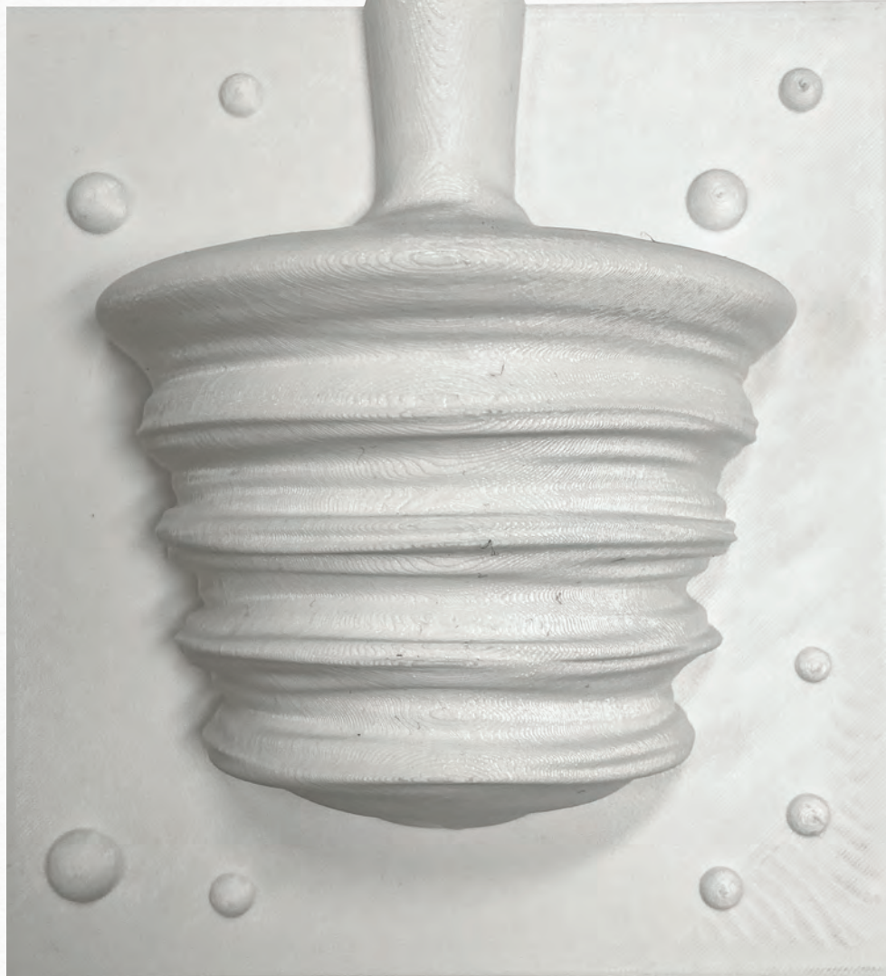
A 3D-printed pot design utilized for creating the plaster master mold.
