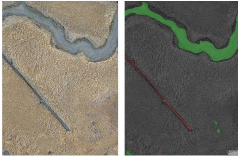
Figure 3. An RGB drone image (left) with its corresponding segmentation map created with LabelMe software (right) where green indicates a non-ditch water feature and red indicates a ditch.
