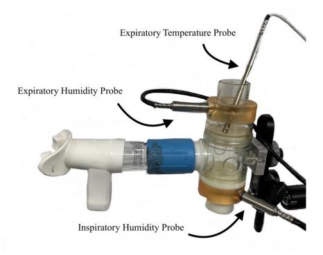
Figure 1. Labeled Hans Rudolph Exercise Mouthpiece. Arrows shown in figure point to probes inserted in the exercise mouthpiece to calculate inspiratory humidity and expiratory humidity and temperature.
