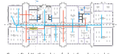
Cross + Stack Ventilation brings fresh air throughout circulation spaces. Ground-based heating and cooling system brings refrigerant through base embedded in walls, allowing for consistent year round comfort naturally, and the ability to simplify interiors to reduce sensory overload, as well as costs.
