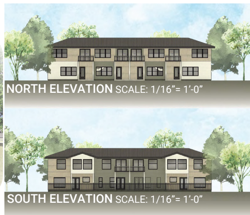
Figure DF.4: Rendering and elevations of the Townhouse A/B housing unit show buildings that could fit into the single-family neighborhood while housing two families. This typology is one of several housing unit options offered in order to increase availability and affordability
