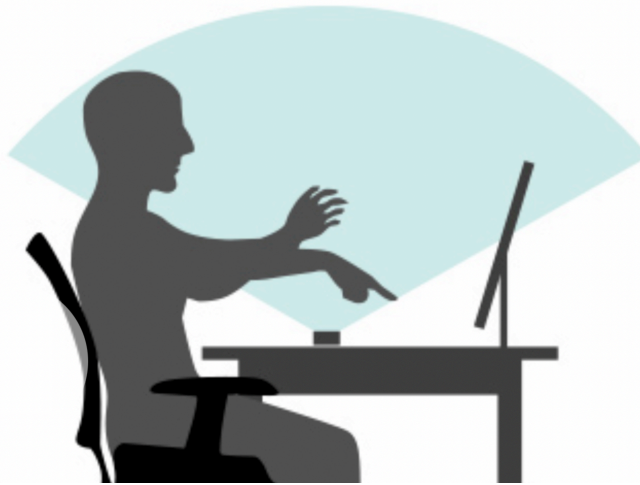
Figure 22. Leap Motion hand-tracking interaction zones
