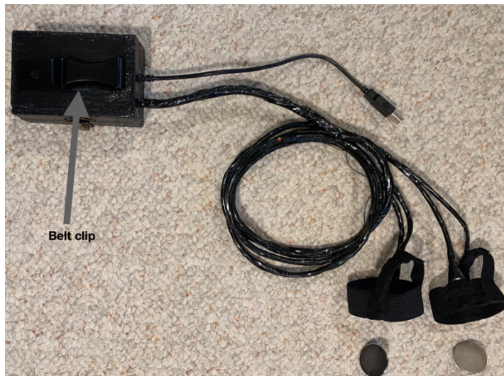
Figure 29. The complete wireless wearable interface
