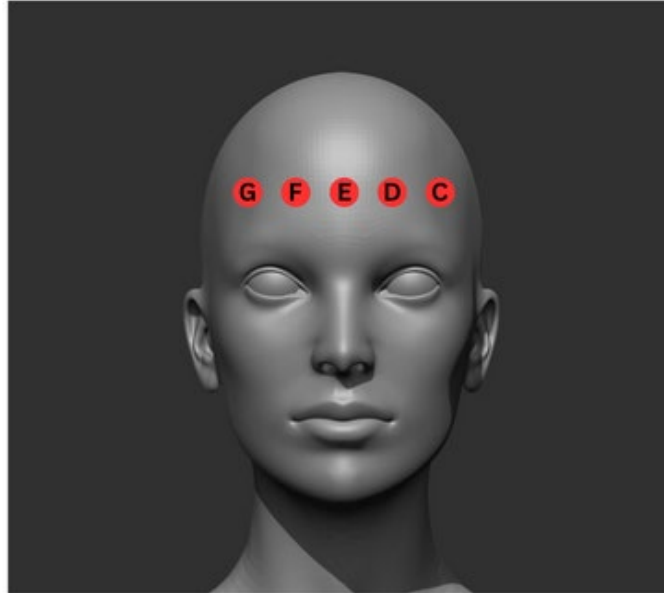
Figure 7: A head model with labeled placement of the vibrotactile nodes on a subject's forehead. Starting from the subject's left, they are labeled C-G. Nodes are placed 1 centimeter apart from each other's edges horizontally.
