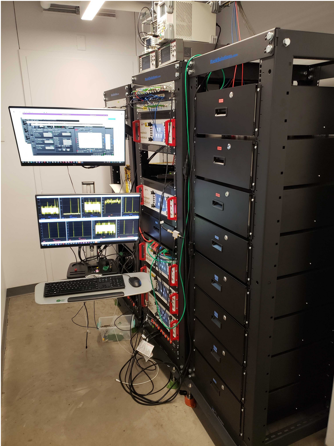
FIGURE 3.6. The laser racks. Contains our breadboard laser systems used for ionization, cooling, preparation, and readout.
