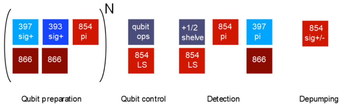
FIGURE 5.2. Laser and rf operations on the ^{40}\text{Ca}^+ Zeeman qubit in the D_{5/2} manifold. The preparation pulse sequence is performed N times, until a satisfactory preparation fidelity is achieved. The qubit operations (using the 976 nm Raman beams) may then be performed while the 854 nm light shift beam is on. To read out the qubit, we first shelve the m = +3/2 population in the m = +1/2 state and then deshelve this population with an 854 nm \pi -polarized laser beam. We then check for population in the S_{1/2} and D_{3/2} manifolds with the 397 nm and 866 nm laser beams. Finally, we can depump into the S_{1/2} manifold with the 854 nm \sigma^- -polarized laser beam.
