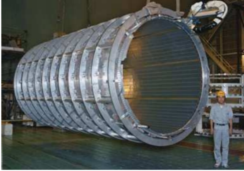
FIGURE 2.8. Central solenoid before installation [8]
