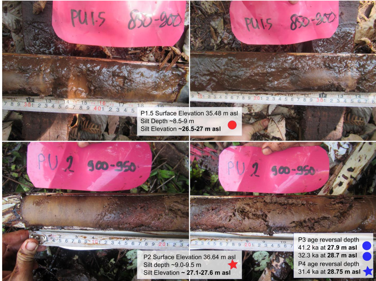
Figure S3.9. Silt deposit in cores P1.5 and P2 and its corresponding position in the peat dome
