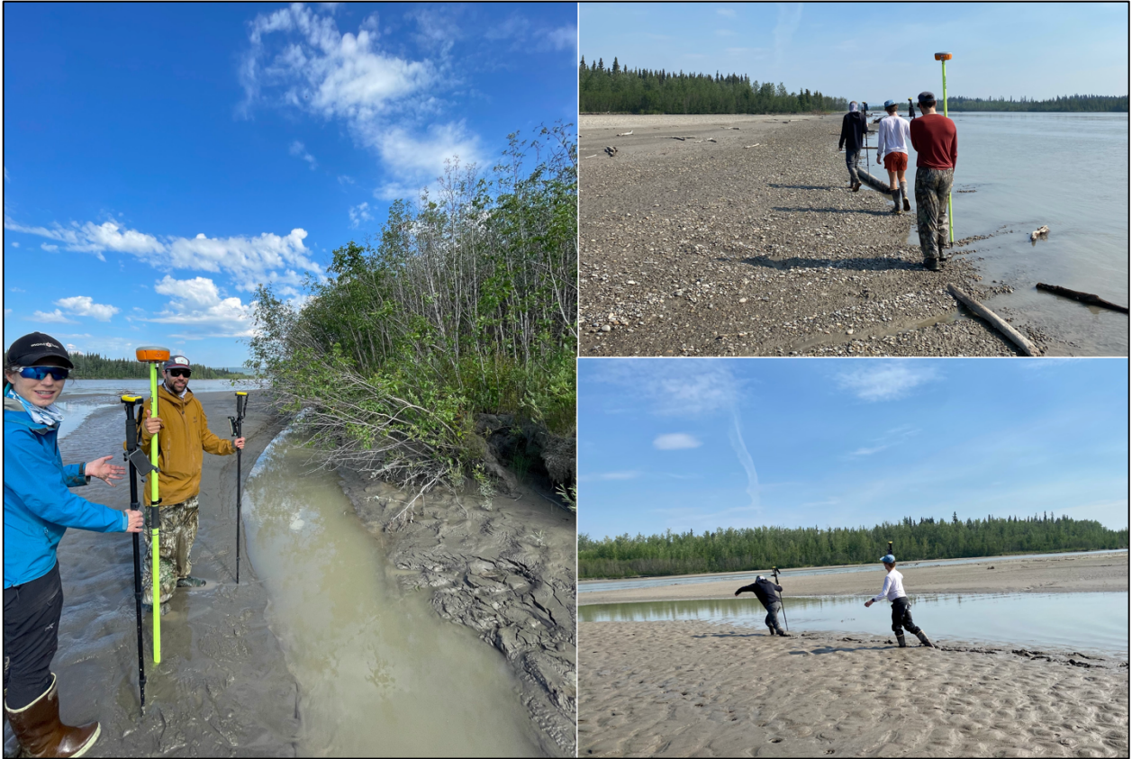
Figure 6. Handheld (black and yellow) and High-precision receivers (green and orange), we had a consistent methodology, including survey poles and walking directly above the wet/dry interface.
