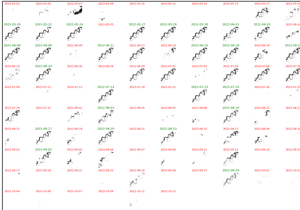
Figure 17 – An adaptive thresholding approach to identify discharge over the Tanana River. This example shows S2 imagery using a subset of dates over the reach of interest. Red days are not included in the analysis due to not enough clear data pixels over the reach.
