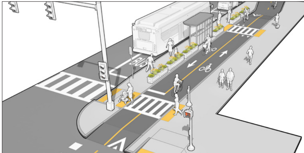
A case study of a floating bus stop that provides a traffic buffer to a two-way cycle track.
