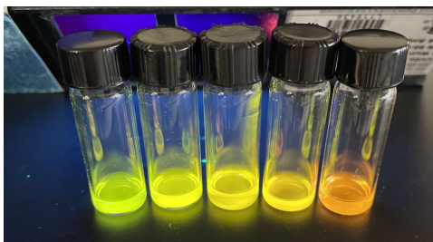
Figure 4.2. BT[11+1]CPP dissolved in various solvents from least polar (left) to most polar (right) and illuminated with longwave UV light.
