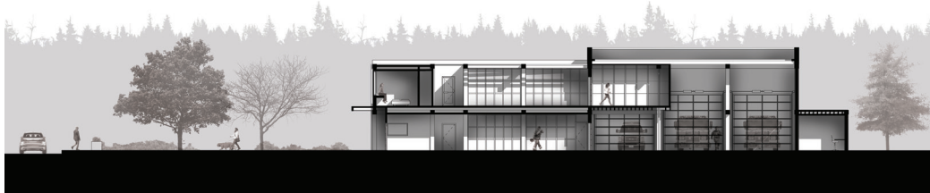
Figure 6: Building section cutting east-west through the site.
