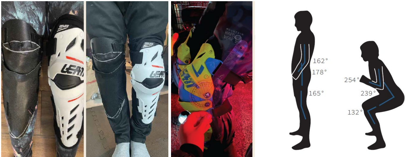
Figure 22: Adjustable hinge prototype left, baseline testing and benchmark joint angles right
