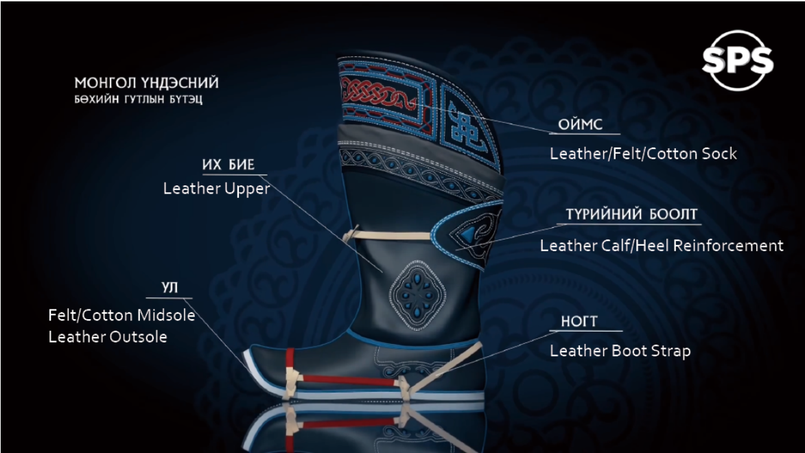
Figure 11. Mongolian Style Wrestling Boot and Components
