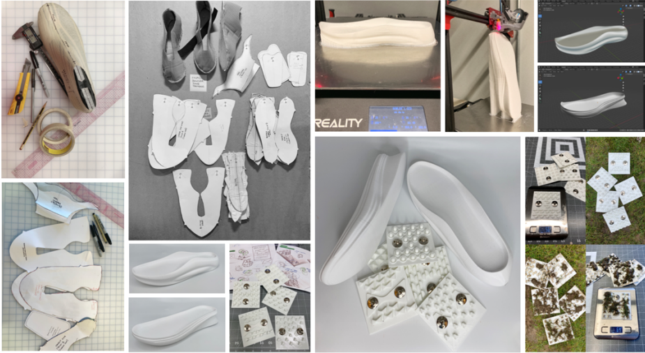
PROTOTYPING (Upper pattern + traction switches + midsole)
