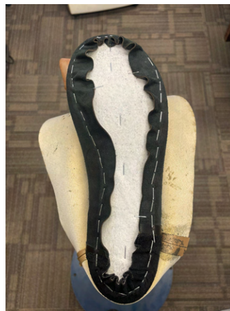
Figure XVI : Initial Fit Check and Stapling Process
