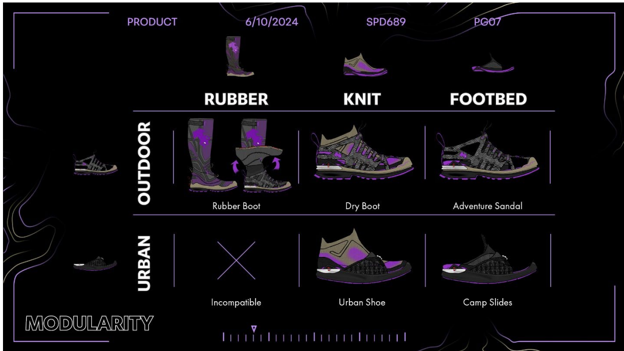
Figure 52 Modularity overview showing which uppers are compatible with which soles to make each piece of footwear
