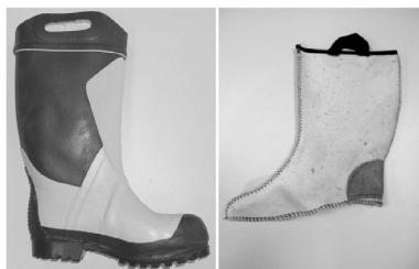
Figure 1. Protective footwear and wool felt liner used during the tests.
