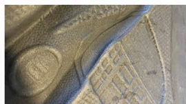
EVA Foam Molded Outsole EVA outsole prototyped using 3D printing
