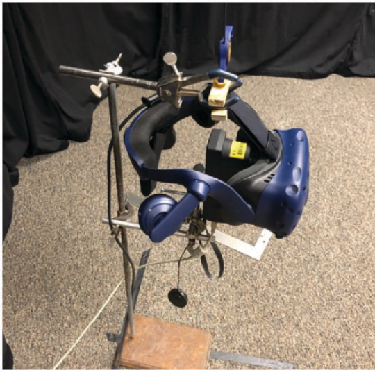
Figure 3. Our spectrophotometer (Minolta CL 500A) mounted in the HTC Vive Pro HMD. This apparatus was rotated to capture readings in 45° angular increments for each lighting condition
